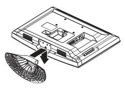
**3** Secure the stand with the three M4 x L14 mm screws (included).
